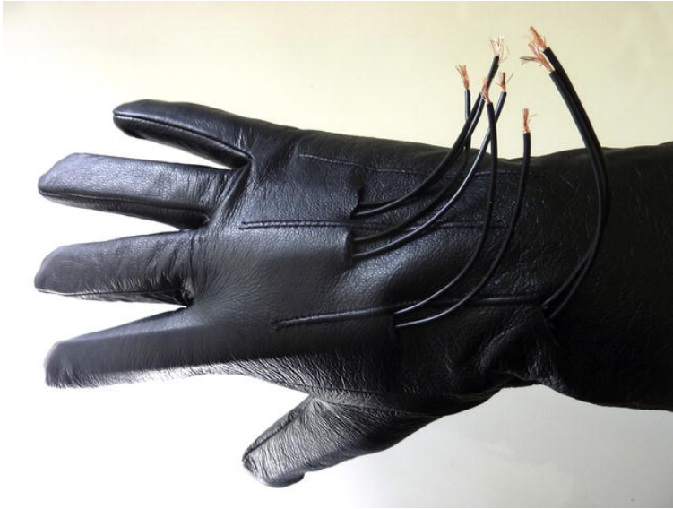
Figure 11-7. Flex sensors installed in the glove
