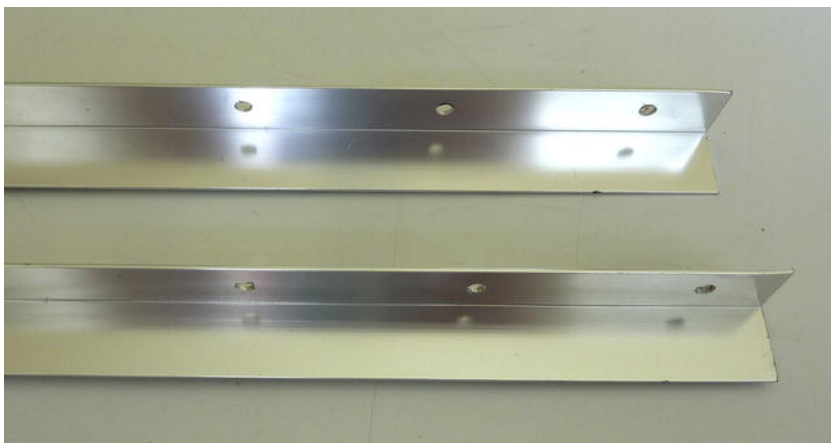
Figure 12-13. Bracing aluminum angles after drilling the holes
