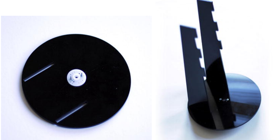
Figure 6-6. Servo arm fixed to disc (left), and robot supports (right)
