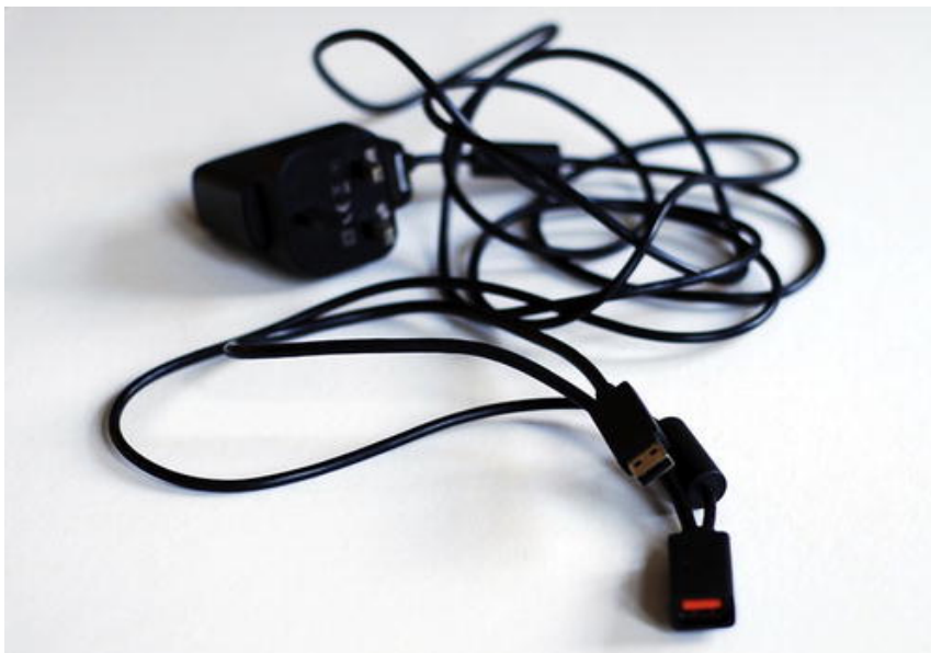
Figure 2-2. Kinect AC adapter with standard USB connection
