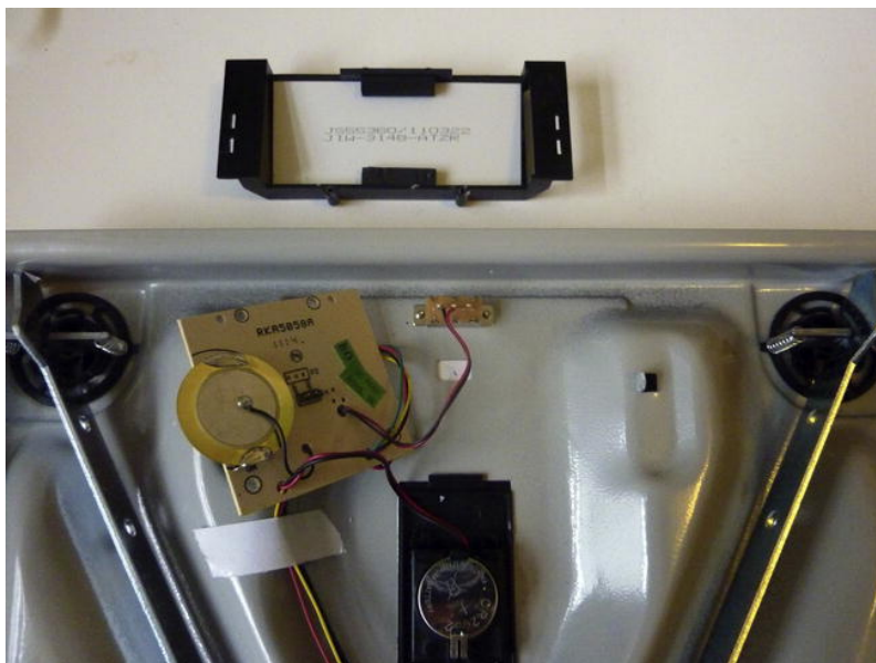
Figure 10-2. Scale after removing the cover and LCD
