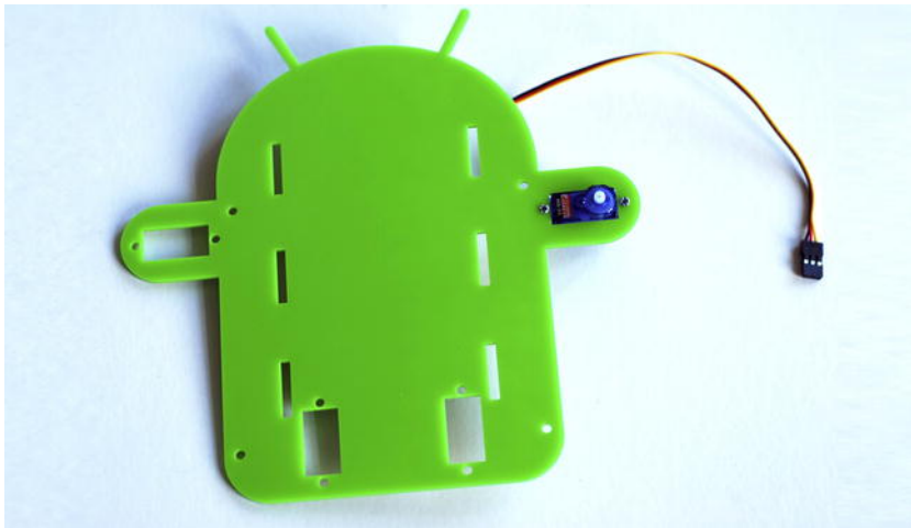
Figure 6-8. Assembling servos to the back body
