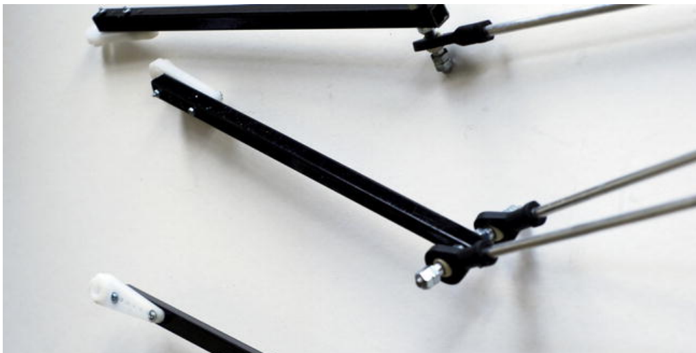
Figure 13-6. Legs ready to be assembled to the base and effector
