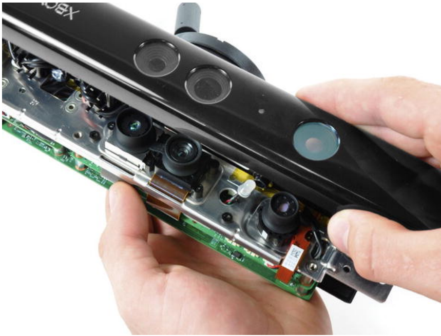
Figure 2-4. Left to right: Kinect IR camera, RGB camera, LED, and IR projector (photo courtesy of ifixit)
