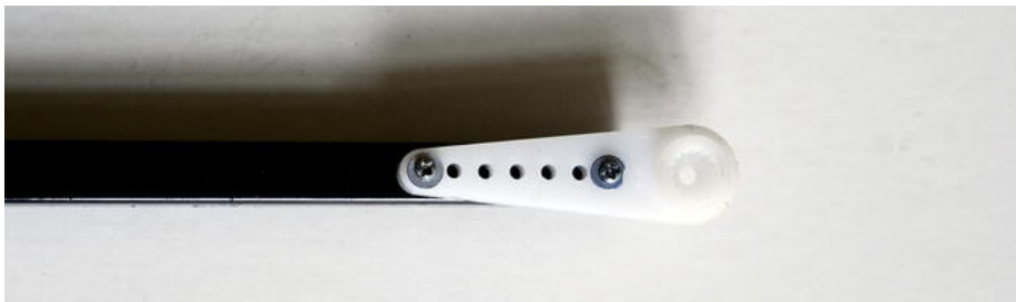
Figure 13-2. Thigh connected to the servo horn
